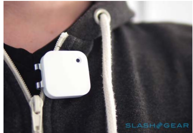
Figure 19 The Narrative clip attached to a vest. This camera takes a photo automatically every 30 seconds. Additionally, photos can be made by double tapping the device.
