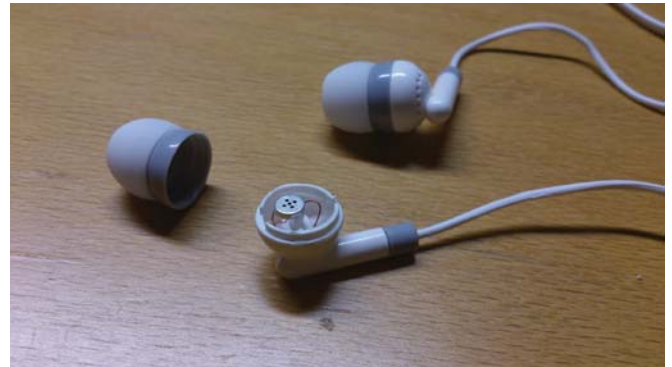
Figure 20 Electret condenser microphones embedded into in-ear phones. The signal output of these microphones, without amplifier, was too low to process.
