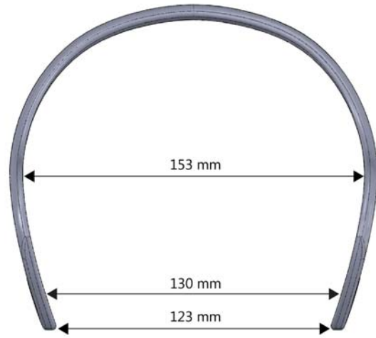
Figure 48 Width measurements of the SW model prepared for mechanical analysis.
