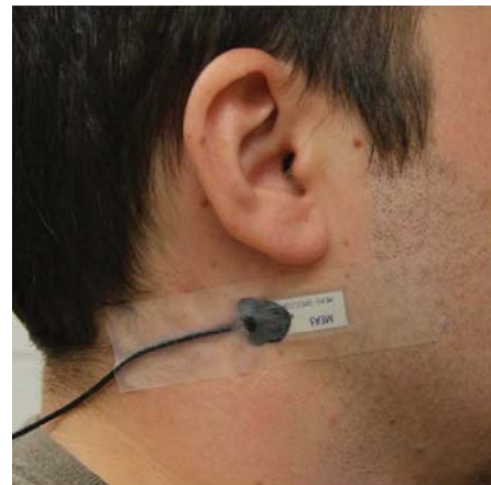
Figure 16 Strain-gauge sensor adhered to someone's jawline in order to monitor characteristic jaw movements for intake recognition (Sazonov & Fontana, 2010).
