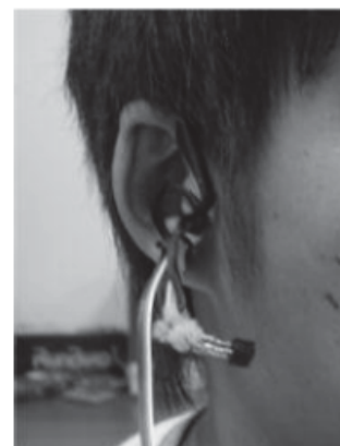
Figure 18 The photo-reflector sensor as used in the research by Kitazono et al. (2011).
