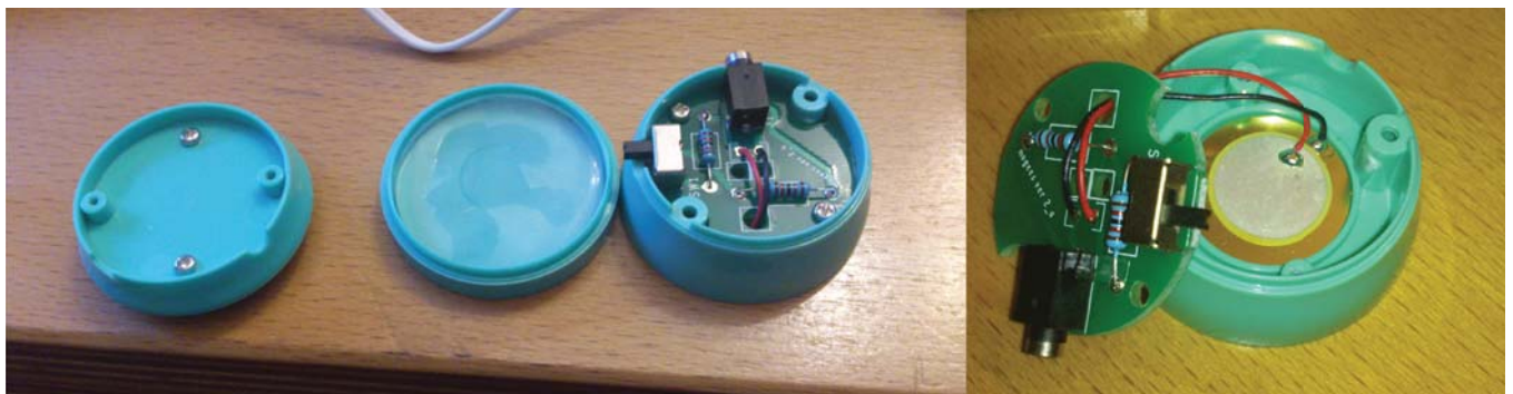
Figure 23 The Mogeess taken apart. The hardware consists of basic components: a piezo, two 12 kOhm resistors, a switch, a PCB, the housing and a sort of gel.
