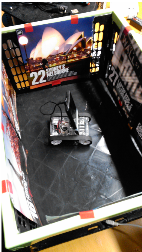
Figure 6-4: Experimental set-up. The robot is equipped with a smartphone and has to learn the relation between actuator and sensor data by rotating and looking at pictures inside a box.
